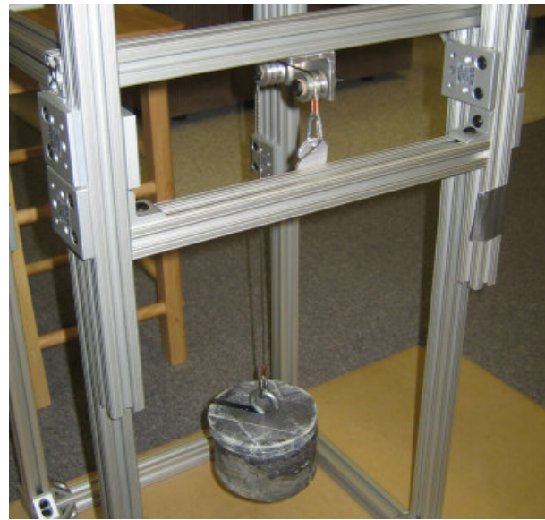
Figure 3: The counterweight system (3D Tractus in the upper position).
