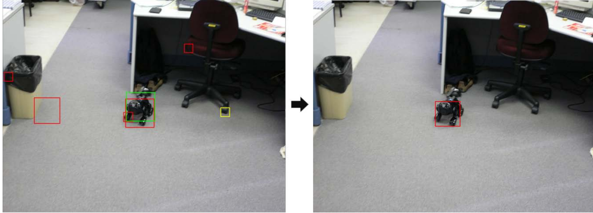
Figure 5: Example of voting scheme. The image on the left represents the results from the various classifiers: red=Top, green=Back, right/left=Yellow, front=Blue. The image on the right shows the resulting match after voting.
