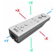
Figure 2. The coordinate system of e Wiimote
