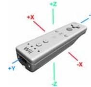
Figure 2. The coordinate system of e Wiimote
