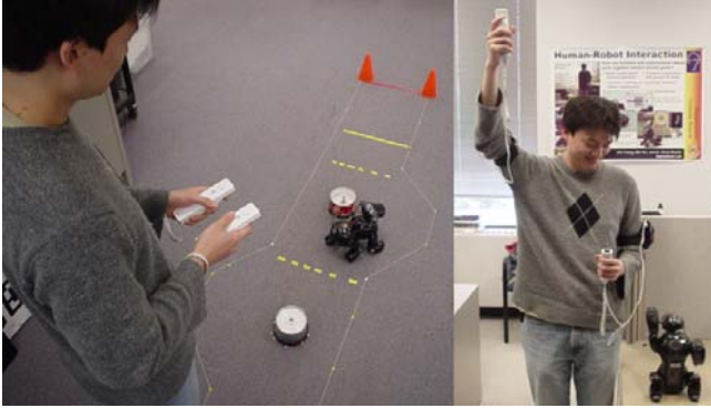
Figure 1. On the left, the user is navigating a Sony AIBO robot dog [7] through an obstacle course using two Wiimotes. On the right, the user is controlling the AIBO to perform a posture using one Wiimote and one Nunchuk on each arm.
