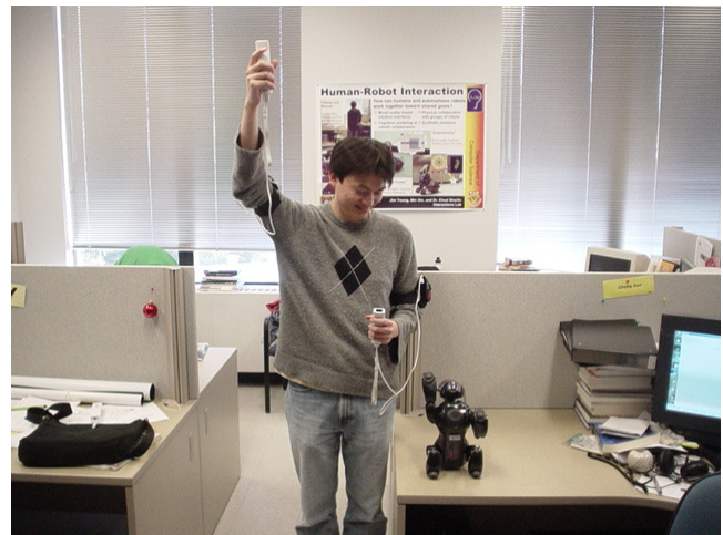
Figure 2. The user is controlling the AIBO to perform a posture using one Wiimote and one Nunchuk on each arm.
