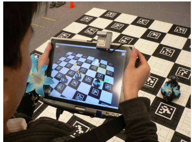
Figure 3: Human player looking at robot suggestions while surveying the mixed reality game environment
