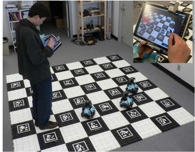
Figure 1: *Sheep and Wolves* collaborative Human-Robot Interaction testbed
